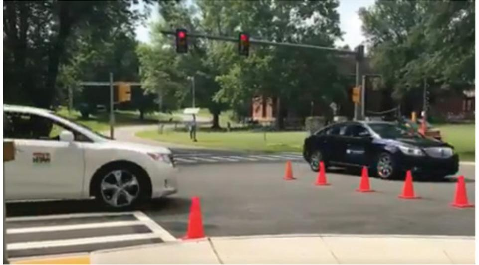
A Tampa vehicle (white) receives an IMA alert while trying to enter an intersection when a New York City vehicle (black) with the right-of-way passes through.
